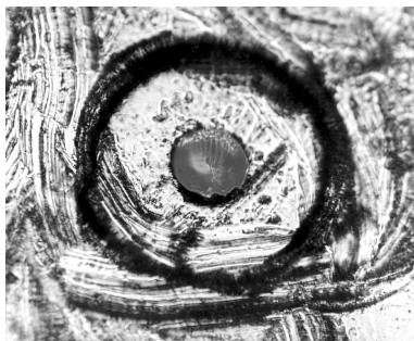
Figure 1-6. Damage from improper cleaning.
